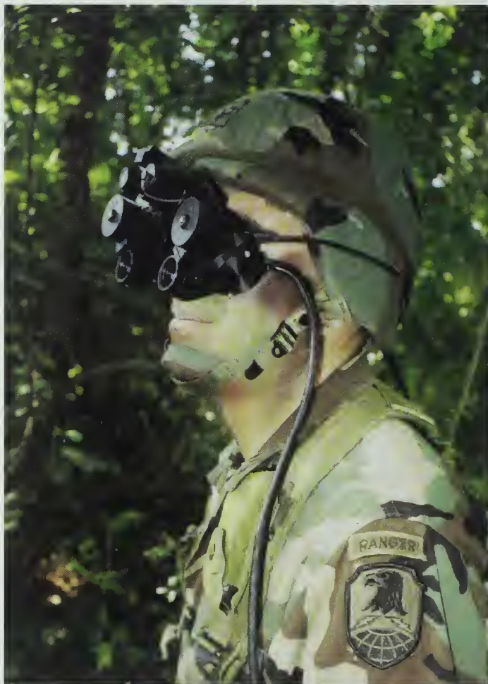
Fig. 6-2. The Uncooled Imaging Technology or UCIT device will enable soldiers to see objects through camouflaje, smoke, fog and other
